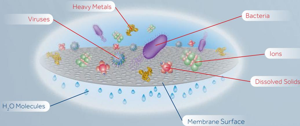
Water pressure forces smaller H<sub>2</sub>O molecules through very tiny semi-permeable membrane pores, which measure 0.0001 microns. This acts as a barrier to contaminants, which are rejected by the membrane and flushed down the drain.
